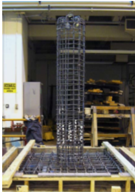
Figure: Details of FRC scale testing cages
